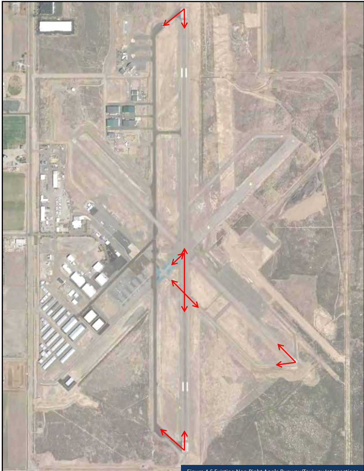
Figure 4-5 Existing Non-Right Angle Runway/Taxiway Intersections
